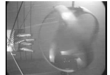
FIGURE 1. Rainbow trout holding Position immediately upstream of the LST at an approach velocity of 5 ft/s.
